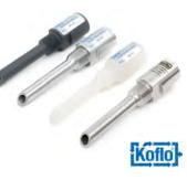
These chemical injection quills feature precision-engineered components, including machined housings that ensure reliable and even chemical dispersion within the center of the pipeline. Each unit comes complete with an integral removable springloaded ball check to prevent flow of the injected chemical into the main flow when the system is shut down.
