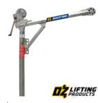
Cranes do not come with base or cable assembly. The cranes use a modular base system to service multiple areas more easily; select from pedestal, socket or wall-mount bases. Cranes also require a cable assembly, choose from either galvanized or stainless steel and with or without a swaged ball. Cable assemblies with a swaged ball can only be used with a manual hand winch, cable assemblies without the swaged ball can be used with either manual hand or electric winches.
