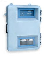
Alarm point is 2 ppm (expressed as mg/L of CaCO3) and is selected by choosing the appropriate model. A rugged, corrosion-resistant and shatterproof ABS plastic case protects the analyzer and reagents. The sealed case is IP62-rated and has a hinged door for easy access to internal components. Easy-to-read LED indicators show a simple "HARD" or "SOFT" sample status. Use the built-in alarm relay to actuate an external annunciator.
