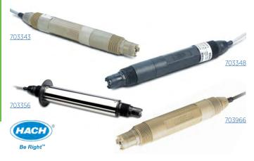
Obtain unsurpassed measurement accuracy, reduced reference junction potential and elimination of sensor ground loops using Hach® differential pH & ORP sensors. These sensors use three electrodes, process, reference and ground, instead of only two electrodes to measure the differential pH/ORP.
