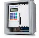
or flow rates. The system can also monitor sound levels, the internal battery condition and detect power failures. The Express II offers temperature sensing across a range from -85 to 300°F.
