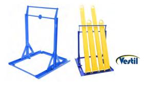
Install or remove fork extensions without lifting, pushing, or getting off the fork truck with a Fork Extension Storage Rack. Simply drive in so tips of forks are over elevated bar, lower forks until they nest in channel in base of rack and back fork truck out of fork retraining straps. Fork extensions not included.
