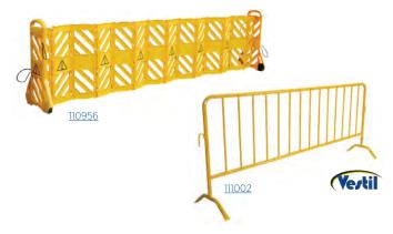
Use these Safety Barriers to close off areas and for crowd control. The mobile, plastic barrier folds easily and is held in closed position with black elastic cords. Simply tilt and roll on two 5" diameter wheels. The crowd control barriers interlock to an expanded length to easily direct personnel. Feet are removable so railing will lay flat for shipping and storage.
