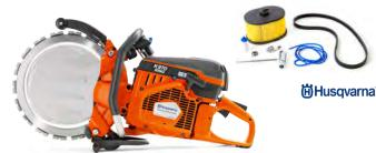
Use the K970 Ring Saw for deep cutting irregular openings in concrete, stone and masonry. The maximum depth of cut is 10", twice the amount of a traditional power cutter. The adjustable water valve makes it easy to ensure dust is reduced while minimizing water consumption and slurry.
