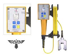
The Raven Sludge Interface Detector is a portable handheld instrument that accurately determines the sludge blanket solid/liquid interface depth in primary tanks, clarifiers, sedimentation basins, lagoons and a wide variety of tanks with settled sludge and solids. The unit is equipped with a strain relieved signal cable with 1-ft increment depth marks and a sensor probe.
