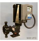
The motor driven BLACKLINE Series MD Pumps feature a spring return mechanical diaphragm for precise and accurate metering control. The oil lubricated ball bearings in an anodized aluminum housing and rugged double-sided PTFE-faced diaphragm provide long service life. Micrometer style stroke length adjuster provides 10:1 turndown ratio manually; select pumps with VFD vector drive to obtain up to 100:1 turndown ratio.
