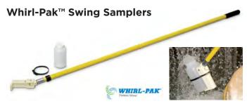
Easily collect samples from a horizontal flowing stream, such as a sewer with the Nasco Swing Samplers. The end of the sampler swings, allowing collection from different angles, including 90 degrees. The 8-ft. adjustable fiberglass pole extends to 12 ft or 24 ft (depending on model) providing a long length for any sampling situation.
