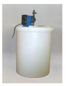
These tapered HDPE Chemical Solution Tanks feature rigid covers that accommodate top mounting of CHEM-TECH 100, 200, most PULSAtron pump models and 1/20-hp flange mount mixers. The covers feature a 4.5" refill cap, 1.4" cap pump accessories and two 3.5" indent for mounting accessories. Tanks are translucent and come with 5-gallon graduations.
