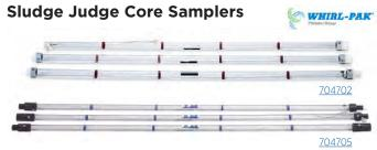
Take accurate readings of settleable solids, 5% or less to any depth with these Sludge Judge Samplers by Nasco Sampling. Samplers are ideal for sewage treatment plants, chemical plants and food processing facilities—anywhere accurate sample levels of settleable solids in noncaustic materials are needed. Each sampler is constructed of durable butyrate tube; a 1-ft (0.31 m) marker on the tubing helps identify the amount of sludge in the tank.
