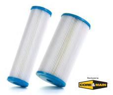
Durable Polyester Pleated Cartridges are durable, washable and reusable. The polyester media pleated around a polypropylene core provide added strength. The ends are immersed in a thermosetting vinyl plastisol which fuses the three components together forming a unified end cap and gasket. The pleated cartridges are bacteria and chemical resistant and provide great dirt holding capacity to extend the time between cartridge change outs.
