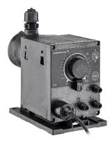
The SMART DDE Digital S and XL Series pumps offer a cost-effective Digital Dosing™ solution with basic functions for simple applications. Unlike pumps that rely on stroke length/frequency adjustment with solenoid drives, the DDE S and XL pumps feature a powerful variable-speed stepper motor with internal stroke speed control for smooth, continuous dosing and impressive turndown ratios.
