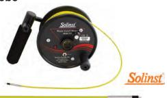
The Model 102 Water Level Meters are designed to measure groundwater levels and are ideal for shallow applications and for accessing very narrow diameters. The included durable P4 probe has no weights and weighs 10 g. When the probe contacts water, the LED light and buzzer are activated. Read the measurement on the cable at the top of the well casing or bore hole to determine the water level.
